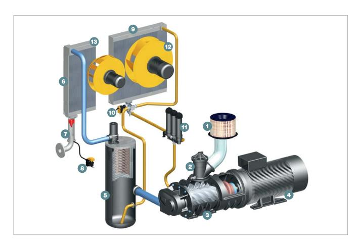
The rotary screw airend (3) is driven by an electric motor (4). The fluid injected primarily for cooling purposes during the compression process is separated once again from the air in the fluid separator (5). The integrated fan ensures cooling of the compressor package and also provides sufficient flow of cooling air through the oil cooler and compressed air aftercooler (6 and 9).
